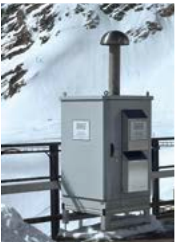
The CS Toptec enclosure from Rittal creates “cosy” conditions for sensitive measuring technology, even in mountainous regions.
